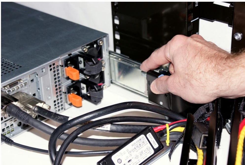
Figure 9: Disconnecting the Inner CMA Attachment Bracket
